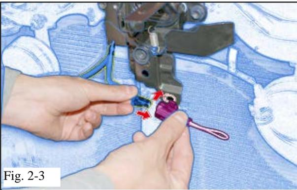
(c) Install the Jumper Connector to the Vehicle's Hood Switch Pre-Connector and attach to Vehicle. (Fig. 2-3)
